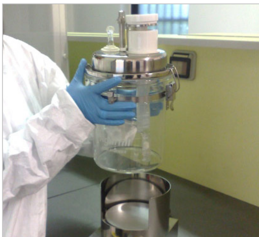
5) Transfer of the Agarfill in the Agarfill System and apply the sterilized tubing and tip to the outlet of the container
