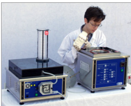
(1) Transfer of the medium into the vessel of Agarster Eco Mini medium preparator
