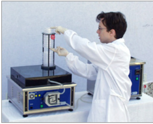
(5) Fill the ADD-MINI petri dish filling machine with standard disposable 90 mm Petri dishes
