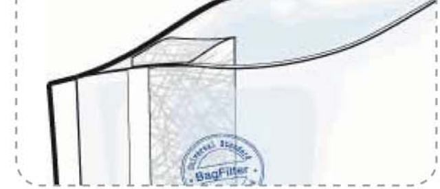
Lateral filter, ideal for fibrous sample
